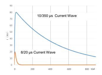
Standard lightning test wave
